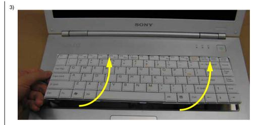
ROTATE THE KEYBOARD FROM THE BOTTOM TO REMOVE
