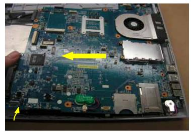
LIFT UP THE LEFT SIDE OF THE MOTHERBOARD AND SLIDE THE MOTHERBOARD TO THE LEFT TO REMOVE
