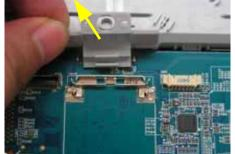
REMOVE ONE SCREW FROM THE LCD HARNESS ROUTING GUIDE. LIFT THE ROUTING GUIDE UP
