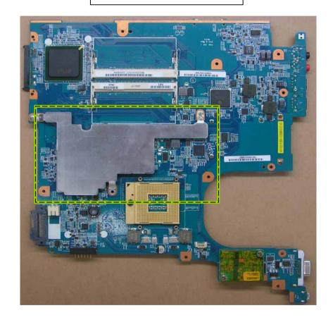
REMOVE TWO SCREWS AND LIFT THE VGA THERMAL UNIT UP
